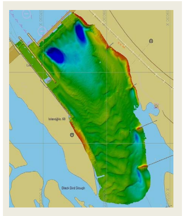
Dual Head Sonic 2020 Survey Lock & Dam Mississippi River
